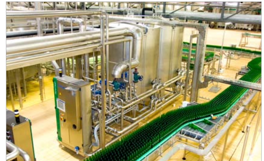
VarioClean in a beer bottling line
