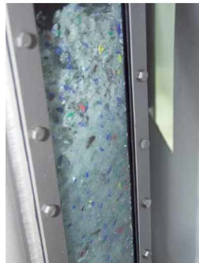
Hot caustic washing
